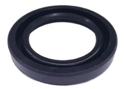
Fabric Reinforced Seals offer similar performance as traditional oil seals, but the lack of metal eliminates issues with rust and corrosion. Damage during installation is avoided and the composite material acts as a gasket-type seal, making it effective when the bore is worn.
